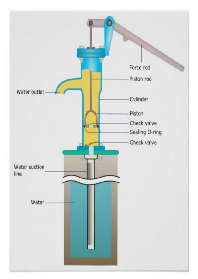
• Pushing the handle (force rod) down lifts the piston and the lower check valve opens and suction brings water into the pump head.
