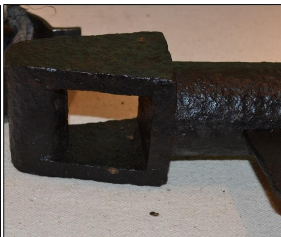
Figure 28: Spalling iron with metal flakes scattered around objects at the Museum of the Iron.
