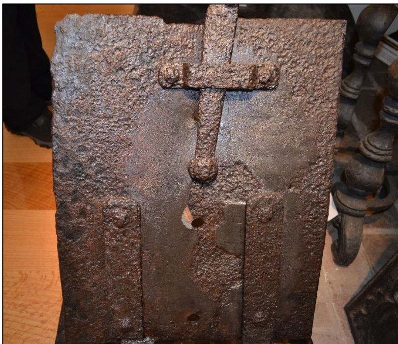
Figure 26: Spalling iron with active rust at center of stove door in Museum of Ironworker.
