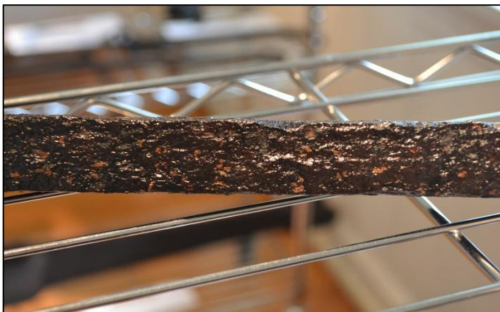
Figure 39: Spalling iron at Museum of Ironwork. Open shelving does not provide even support or security for object.
